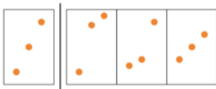
Figure 3.5: Same ordinal pattern of order d = 3 (left) for three different motifs (right).
